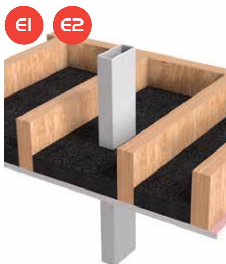
FZ100 Fire Safe Zone and PVC duct
