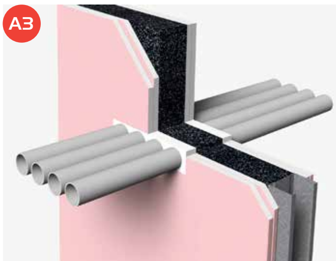
FZ100 Fire Safe Zone and combustible pipes
