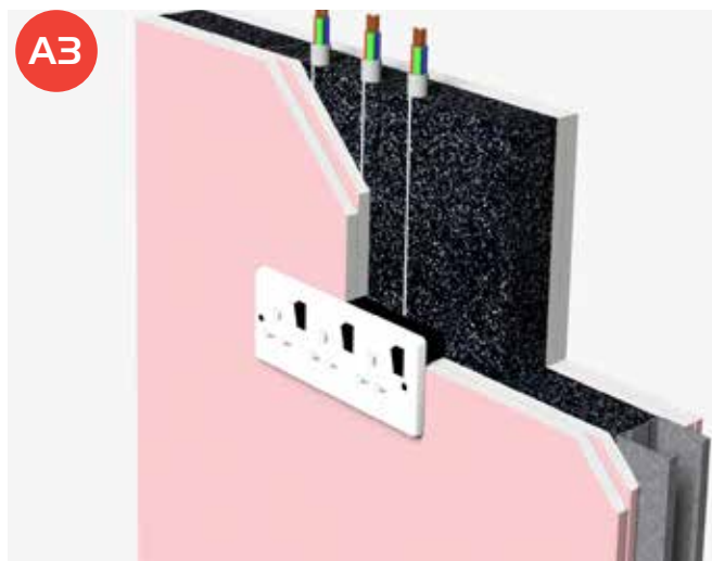
FZ100 Fire Safe Zone and gang socket box with twin and earth cables
